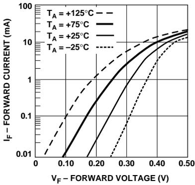
Figure 1. Forward Current vs. Forward Voltage at Temperatures.
