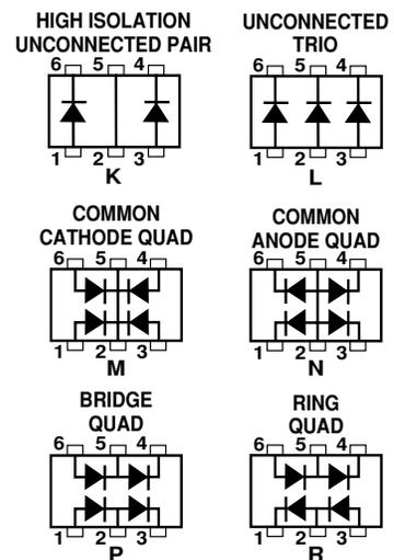
HSMS-282x series of diodes is the best all-around choice for most applications, featuring low series resistance, low forward voltage at all current levels and good RF characteristics.
