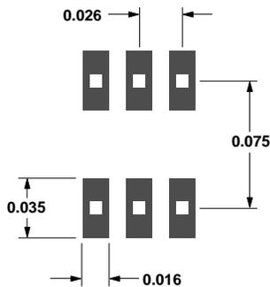
Figure 27. PCB Pad Layout, SOT-363 (dimensions in inches).
