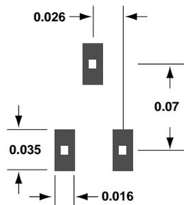
Figure 26. PCB Pad Layout, SOT-323 (dimensions in inches).
