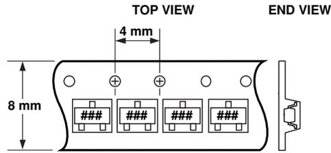
Note: "###" represents Package Marking Code. Package marking is right side up with carrier tape perforations at top. Conforms to Electronic Industries RS-481, "Taping of Surface Mounted Components for Automated Placement." Standard quantity is 3,000 devices per reel.
