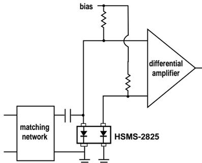
**Figure 13. Differential Detector.**
