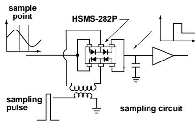
Figure 25. Sampling Circuit.
